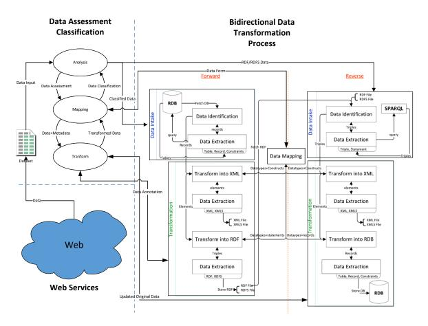
Figure 3. Complete Bidirectional data transformation procedure for e-assessment
